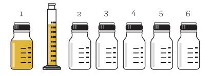
3. Using a syringe, add isinglass at a range of rates. Invert to mix. Leave to settle for 24 hrs. at cellat temperature (10 -15°C).
