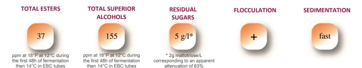
Fermentis dry brewing yeasts are well known for their ability to produce a large variety of beer styles. In order to compare our strains, we ran fermentation trials in laboratory conditions with a standard wort for all the strains and standard temperature conditions (SafLager: 12°C for 48h then 14°C / SafAle: 20°C). We focused on the following parameters: Alcohol production, residual sugars, flocculation and fermentation kinetic.
